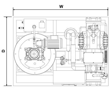
Production capacities based on 25°C condenser water and 16°C sea water temperature Evaporator temperature -28°C Condensing temperature 36°C Ice thickness 1.5 - 2.2mm
