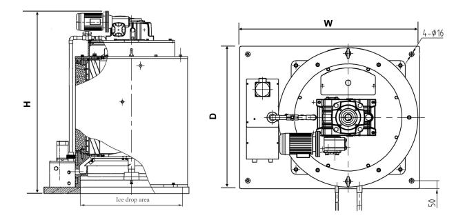
Production capacities based on 25°C ambient and 20°C water temperatureEvaporator temperature -20°CCondensing temperature 40°CIce thickness 1.5 - 2.2mmKater temperature 0-40°CAmbient temperature 5-40°CWater temperature 0-40°C
